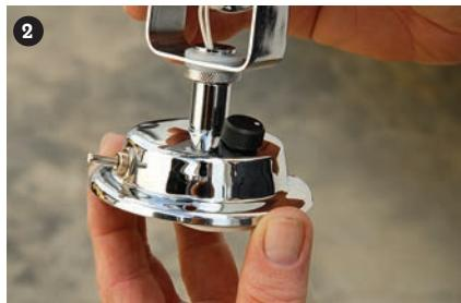
**[1]** Installation requires connection of 12-volt DC positive and negative wires. Don't rely on color coding; check polarity of power leads before butt connecting wires. **[2]** Caribbean Reading Light has metal on/off rocker switch and rheostat to adjust intensity of the light, a feature which gives users better control for reading in bed.
